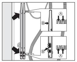
■ Secure the shipping rods to the back of the washing machine. Make sure that the holes
